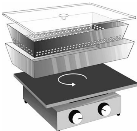
Fig. 6.2: Staining of multiple large format gels on an orbital shaker. Up to four gels, with or without film-backing can be stained together in one set.
