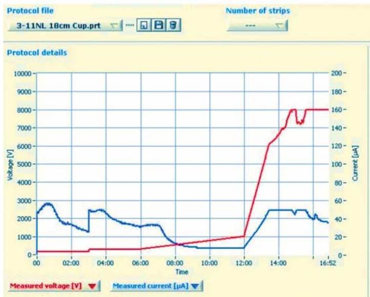
Fig. 1.30: Monitored voltage and current graphs from two IEF runs in IPG strips. For more details see text.
